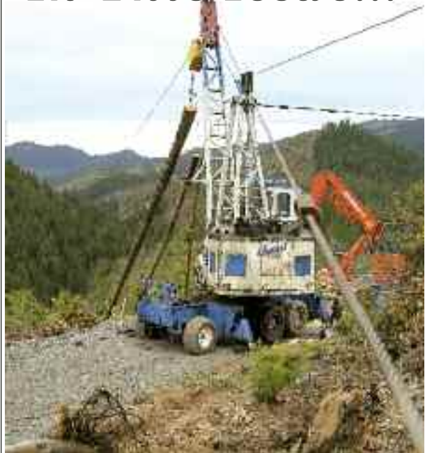
FRONT COVER PHOTO: GT3 YARDER ENGINEER CALVIN TUCKER pulls a turn into the landing with Estremado Logging's Acme 23 motorized carriage as Dan Estremado waits for the turn to land so he can clear the chute with the Doosan DX300LL shovel with Rotobec grapple. Estremado Logging has two GT3 swing yarder sides and a single ground side.
