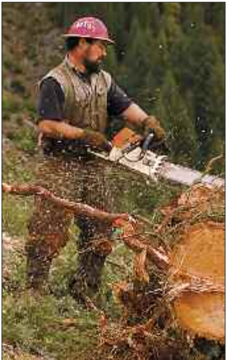
MATT PIRNIEE is the chaser and has been logging since starting with Estremado two years ago. "I love it out here," he said with a smile. He's bumping knots on an oversized tree with a Stihl MS460 Magnum with Oregon bar and chain.
