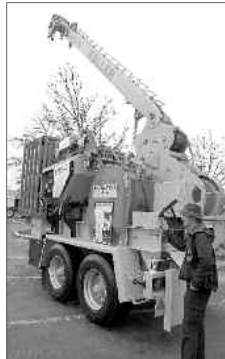
KOLLER NORTH AMERICA introduced their remote control 602 yarder designed for two-man operation at this year's OLC, which has a range of options available.
