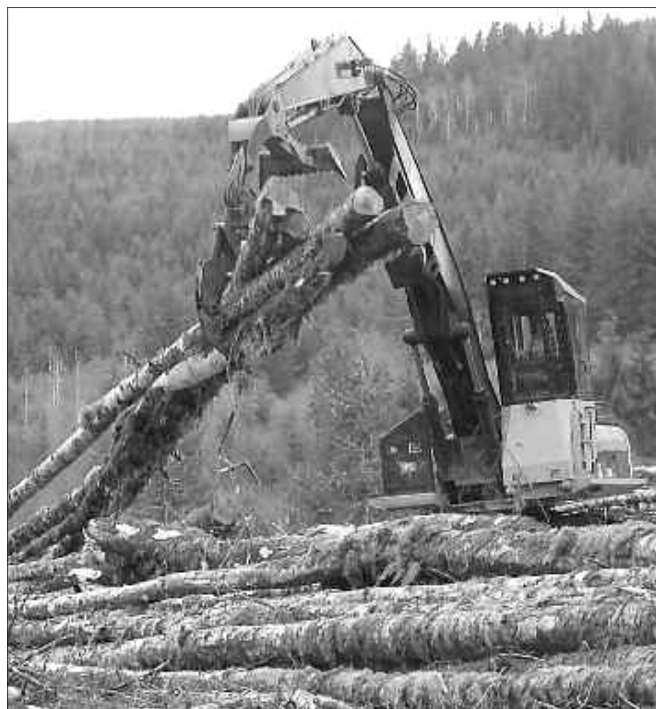
CHARLES HARTMAN shovel logging with his Caterpillar 330D shovel logger, with Cat grapple. "The first pmr we got in '05 when we bought this machine. They talked me into trying it and it turned out we liked it. They roll the logs up real nice," he explained, "and you can grab a bite and keep them straight to load."
