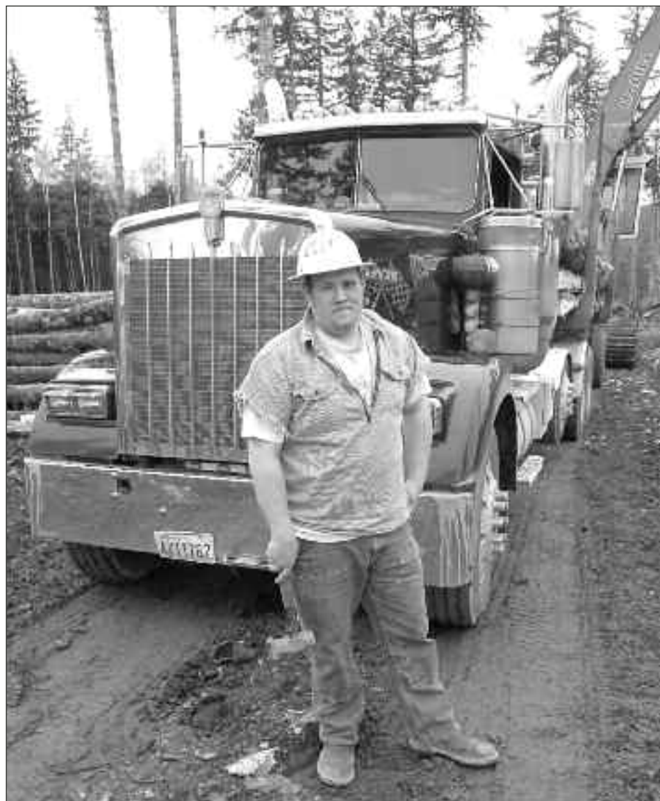
MITCHEL BARNES drives the No. 2 Elliot truck, a '99 Kenworth W900 with a 500 Caterpillar 3406E power plant and a '96 Peerless trailer. He's been driving log truck the past two years braking in working for an uncle in Ketchikan, Alaska, "...and that's how I got started," he explained. "I used to drive the 100-ton 777 Cat haul truck," at an open copper mine in Arizona. "It's just like driving an automatic car," he said, noting it was huge. "The tires, I could stand at eye level and be the middle of the rims. It's a pretty cool machine (he's 6 ft)... 23 miles /hour seems like ur doing 60."
