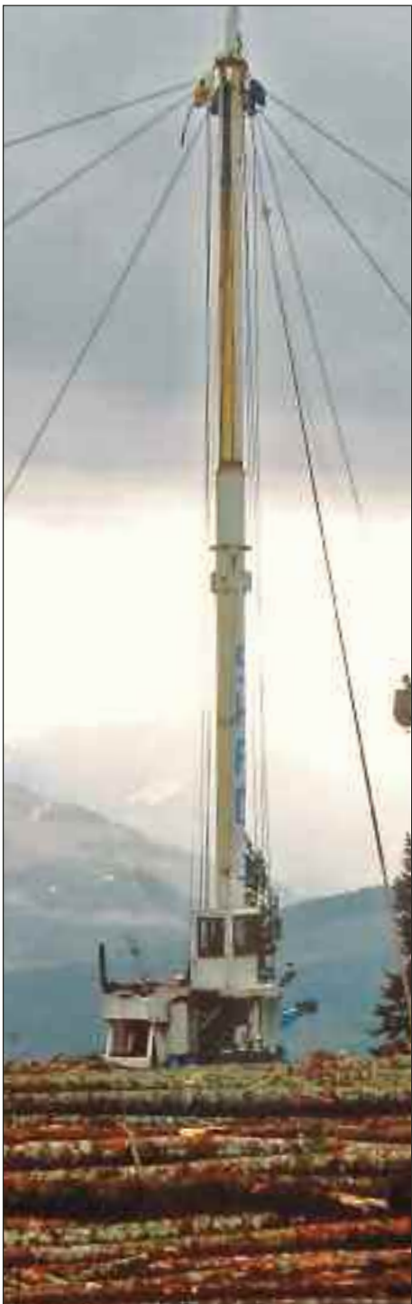
"PRECIOUS" is the name given by Scott Zender to the Zender & Wilburn Skagit T90 tower with BU94 conversion, which they made in 2004 from the original BU80 yarder.
