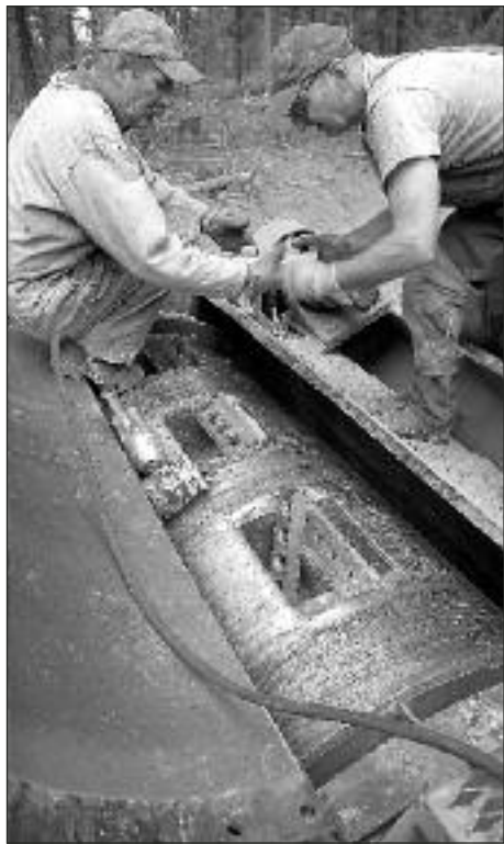
REPLACING THE KNIVES on Medici's Morbark chipper are mechanic Tim Kirby and operator Mark Johnson.
