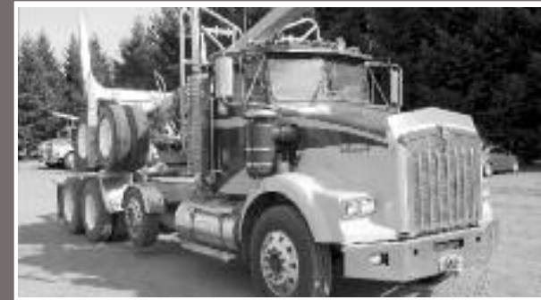
1998 KW T800 , Cummins N.14, Jake brake, 18spd trans, RTLO 18718B, single spd Eaton rear ends, DS 461P w/locker (4:11), Hendrickson walkbeam haul-max, rubber pads, 3/8 steel frame, 251" wheel base, 4-axle truck. Whit-Log trailer w/electric scales $51,500 Office 541-863-5241 • Cell 541-863-1500 X
