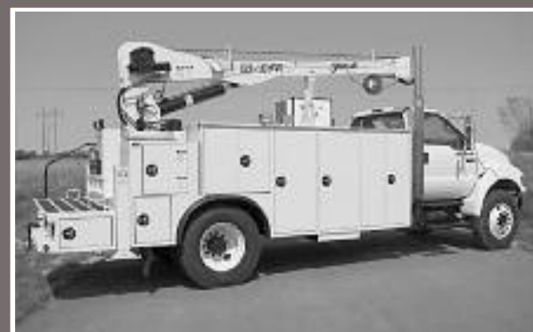
NEW**2010** F-750 Ford, 450 miles, 285 HP Cummins, 6spd trans, new 14' HD crane body, 40 CFM hyd compressor, 10,000lb hyd crane w/wireless controls. Call toll free 855-498-0610 Jack Harriman v
