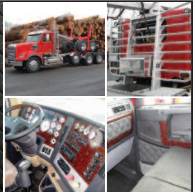
ALWAYS UP FOR A CHALLENGE, Todd Stoffel drives a super-train for Chilton Logging. The truck is a 2005 Kenworth T800 powered by a C15 Cat 550hp motor and equipped with Hassell bunk gear and a Peerless pup trailer.
