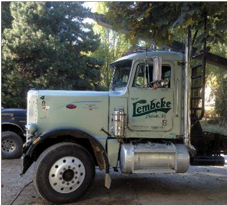
CLINT LEMBKE'S NEWEST TRUCK is a 1981 Peterbilt 359 with a 3406 Cat motor, and Eaton 13-speed. Lembke, who trucks out of Colville, Washington on the Eastern side of the state, writes that the truck was hand painted by John Race when he got it, "but my wife said it was ugly, so I named it Ugly Betty. The other saying was on the hood so we left it cuz it's right -- a bad day hauling logs is better than a good day in jail."
