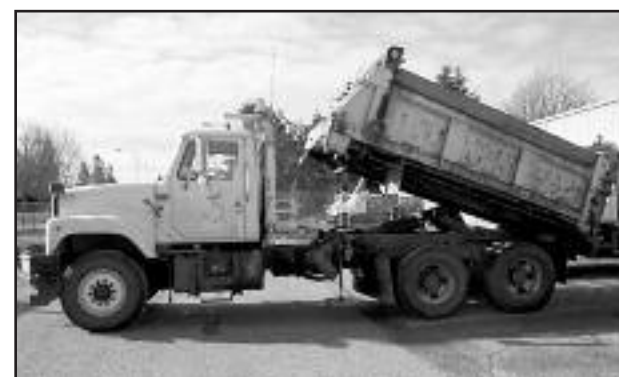
(2) 1998 IH 2574, M-11 plus Cummins, 18-speed, 18K front axle, spreader dump box, Low Miles .....SELLING COMPLETE
