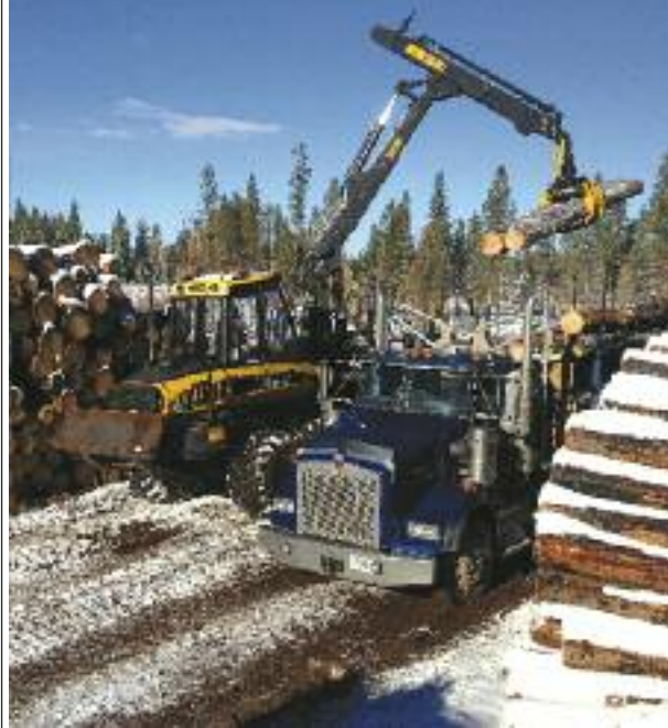
COVER PHOTO: L&L INC DOES A LOT WITH A LITTLE. The southern Oregon logging and trucking outfit utilizes mechanized harvesting and a self-loader for increased efficiency and versatility.
