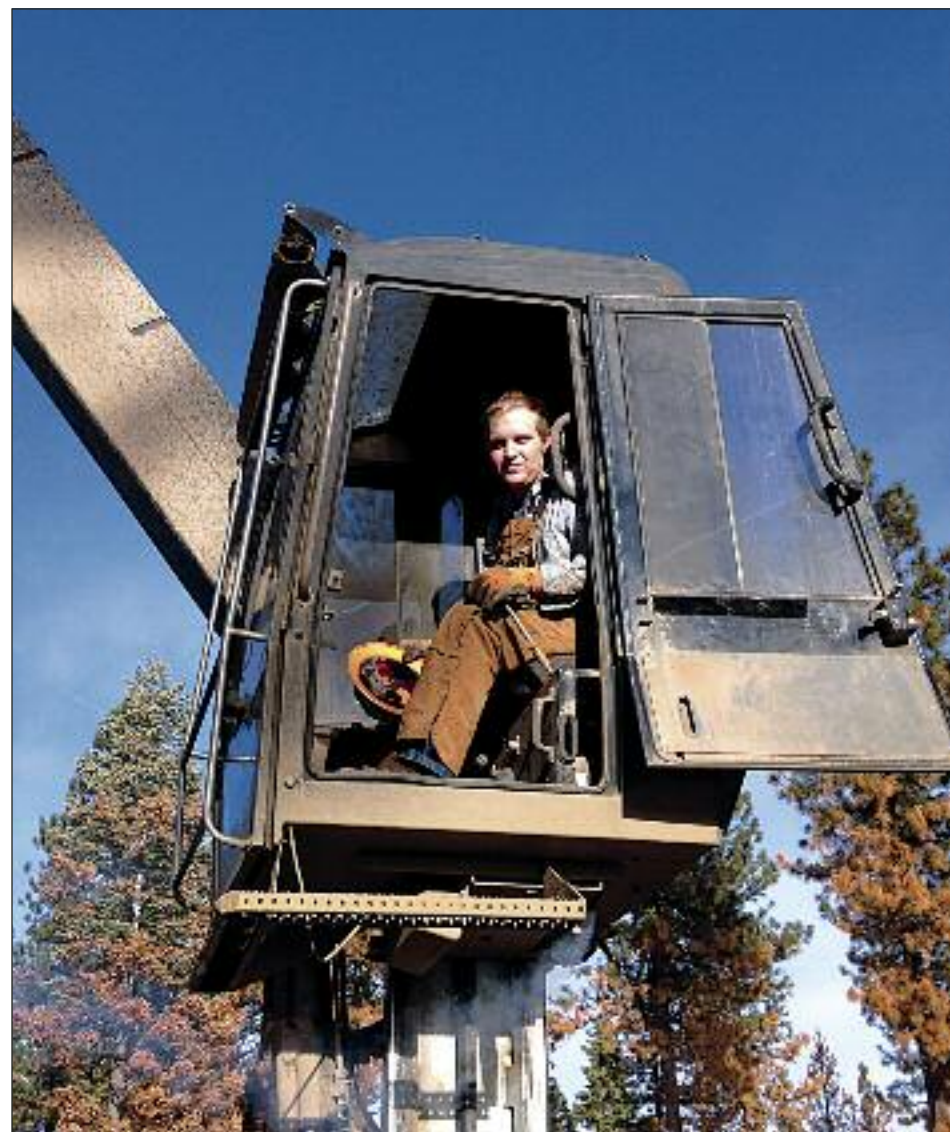
THE ENCLOSED CAB on the Loglift self-loader means increased safety and comfort for the operator Ted Mann.
