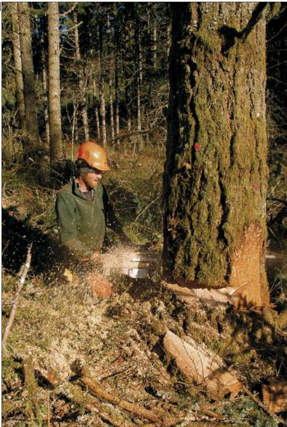
BUCK LOMMEN was cutting the oversized and challenging ground for A-1 seen here using his Stihl MS461 with 36" Stihl lightweight bar and Oregon chain, noting, "...they're stiff for a light bar." This is the second MS461 he's had explaining, "It like it. It's a good saw." He's been a timber faller the past 13 years, and contracting on his own the past eight years. He credits Butch Walty, who he'd worked for years ago, for teaching him the trade.
