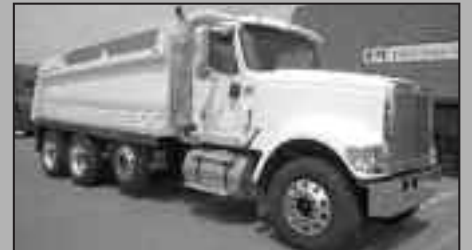
2006 INTERNATIONAL 5900i, ISC Cummins, 475 hp, Jake, 18 speed, 14,600# front, 46,000# rear, air tag, 16' Tub Body, plumbed for pup STK. #4642
