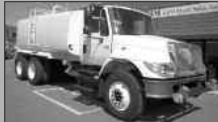
LOW LOW MILES, 2006 INTERNATIONAL 7400, DT466, 250 hp, RTO8908LL 10 speed, 14,000# front axle, 40,000# rear axle, Hend walking beam, 2012 UNITED 4000 GALLON WATER TANK, 2 front, 2 side, 2 rear sprays, self-loading, hose reel, cab controls STK #4600
