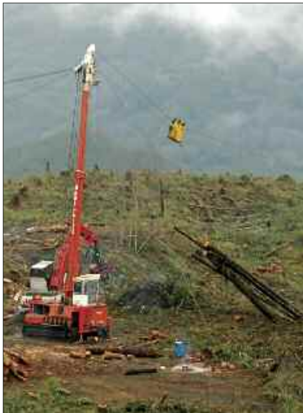
THE MADILL 172 brings a turn to the landing with the Acme 28S motorized carriage. They were hanging out almost 3,000 ft. Chip Cooper is the yarder engineer.
