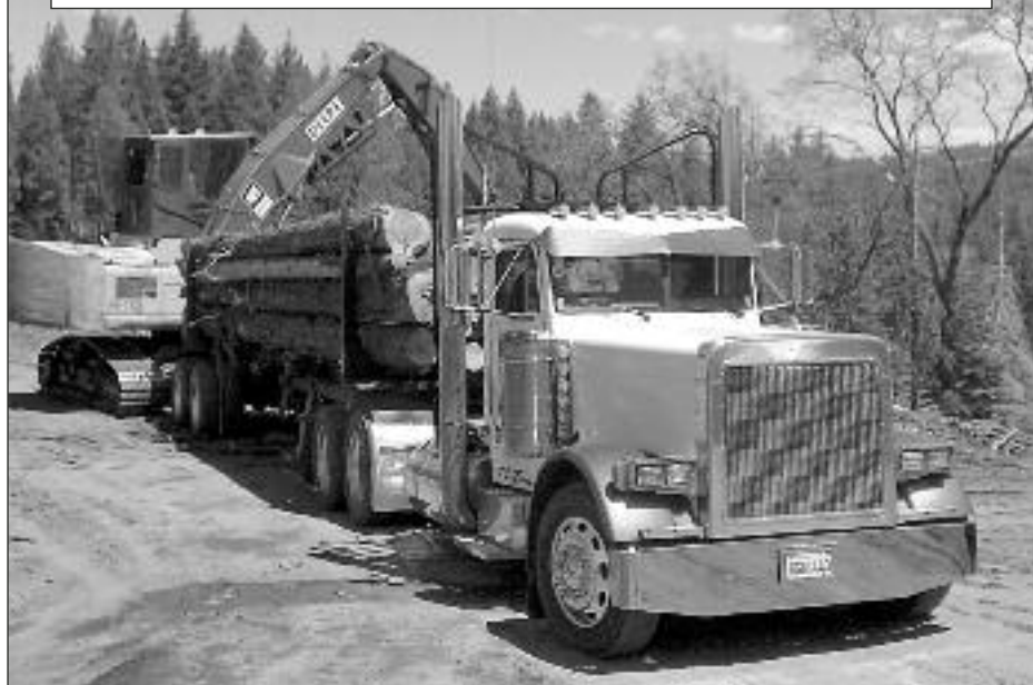
ZAC HAULS LOGS WITH HIS "DREAM TRUCK" - a 2002 Peterbilt 379 extended hood. The truck is equipped with a 600 Cat motor, 18-speed transmission, super 40 double lockers, 3/8" frame, electric scales and a 2000 Hassell conventional log trailer.
