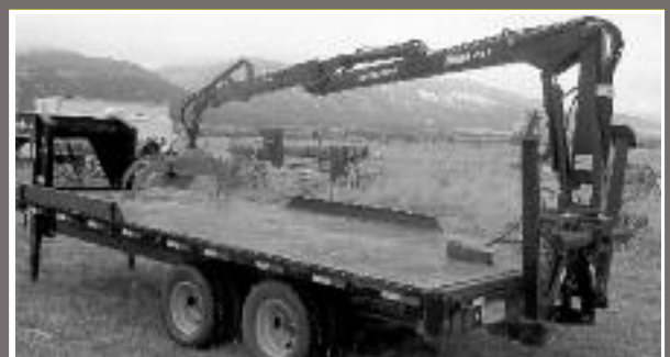
NOKKA 4166 Log Loader , used only for demos, equipped with Nokka 16 grapple, NR3 rotator, fold down legs, tree point hitch and a-frame, max lifting capacity 3,520lbs, min hydraulic output 10.6gpm, weight 1,995lbs. NEW PRICE! 1-800-566-0690 or sales@hakmetusa.com E
