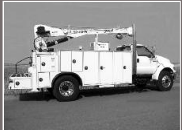
2013 Ford F-750 , 300hp, Feterl body & crane, 40 CFM air compressor, concealed door hinges, LED lights 855-498-0610 X
