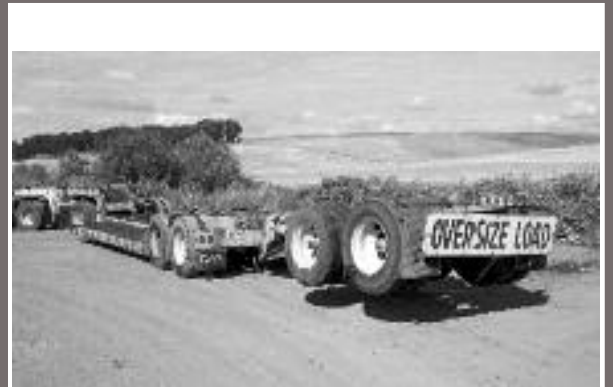
1977 General Lowboy Trailer, 60 ton 2 axle trailer, 9'w x 21'6" well, 30 ton 2 axle Jeep, 2 axle booster $50,000 503-662-3551 F
