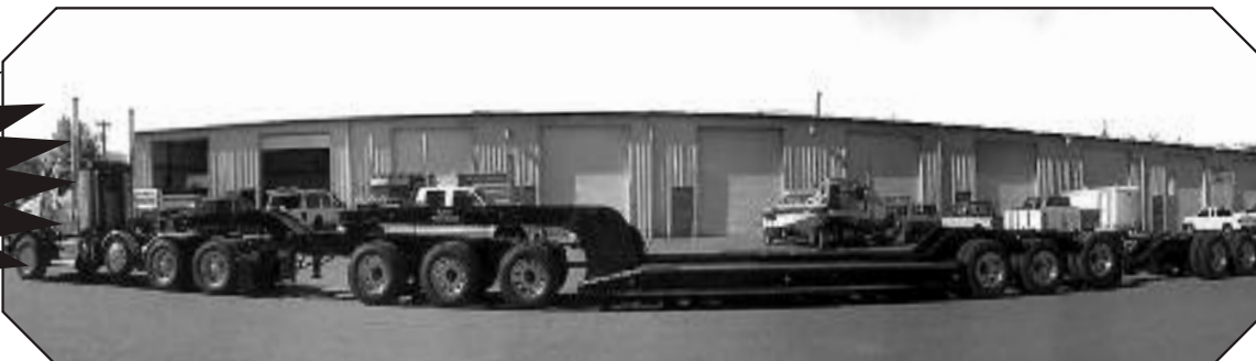
Tyler Picknell Trucking, ROSEBURG, OR, Brand New 2013 Whit-Log 3 Axle All Air Ride Jeep, 80 ton 3 Axle Lowboy, and 2 Axle Booster, Thanks Tyler and Lawrence!!
