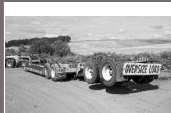
1977 General Lowboy Trailer , 60 ton 2 axle trailer, 9'w x 21'6" well, 30 ton 2 axle Jeep, 2 axle booster $50,000 503-662-3551 G
