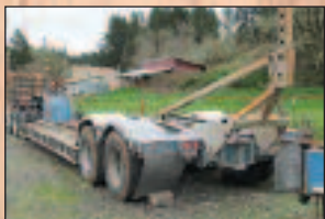
79 GENERAL 50 Ton Lowboy , 9' wide, 21' well, ground bearing, need wet kit, 3rd tag axle (removable), boom stand, outriggers, NEW PRICE. $20,000
