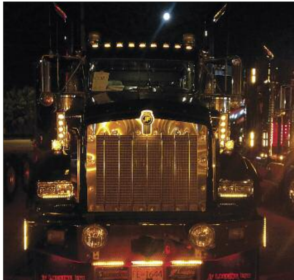
THERE'S NO MISSING THE TRUCKS belonging to J.F. Logging with their abundance of lights. "We go with LED lights because they're brighter, don't burn out and require less maintenance," owner Jed Fryer says. "The driving lights we use Sirius HID drive lights."
