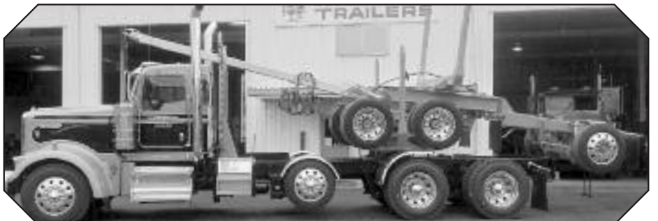
P.E.R. Inc., ELMIRA, OR, Brand New 2014 SE100 Long Logger with a TRD100 3rd Axle Booster and Matching Truck Equipment. Custom Rectangular Tube Cab Guard, Side Step Box, Whit-Log Lift Axle Fender Kit, Double Tapered Stinger, and More. Thanks Ryan & Bill!!
