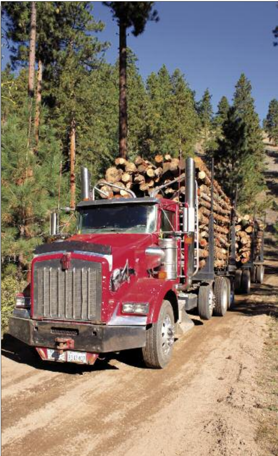
KENWORTH T800 EQUIPPED with an 6NZ C-15 725hp motor, 18-speed transmission and double locker 46's on Chalmers suspension.
