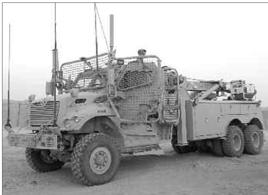
IT'S NOT A LOG TRUCK, BUT RYAN RONNING certainly hauled some heavy loads with the 2012 International MRAP Wrecker he drove while deployed with the ARMY in the Middle East. The armored wrecker is outfitted with a 30-ton rotator, one 50000lbs drag winch and two 25,000lbs lift winch's, part time 6 wheel drive, two speed air shift T-case, five speed Allison trans, Eaton rear ends with lockers in all axles, only 375HP but geared very low, and on board fire fighting gear mini fridge and a microwave.
