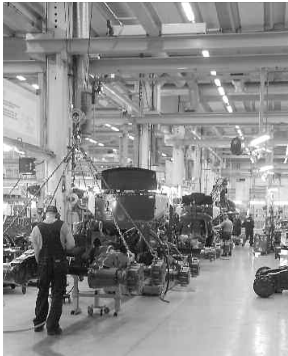
PART OF THE PONSSSE ASSEMBLY LINE in Vierema, Finland was full from start to finish with advance orders well into the future. They follow a "lean manufacturing" model typical of most quality manufacturers for better economy, and higher quality control.
