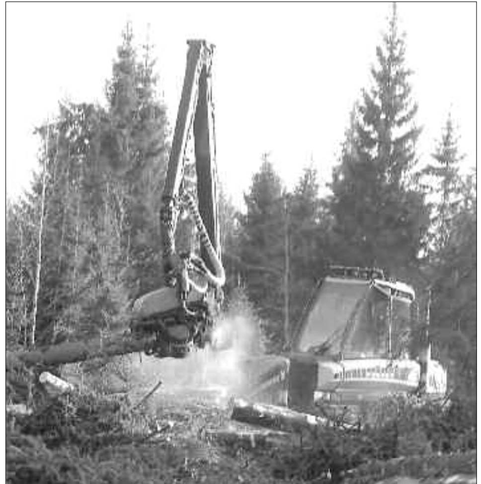
PEKKA AIRAKSINEN cutting and processing logs with the Ponsse Beaver with H6 harvesting head mounted on a C22 squirt boom, works with Otto Piironen who was operating their Ponsse Elk forwarder on the same site. The contractor, FinnHarvest Oy and Piioiset KY, on this UPM managed site, is located near Kupio. The contractor owns 19 Ponsse machines, consists of the eight Piioiset brothers and 25 employees.
