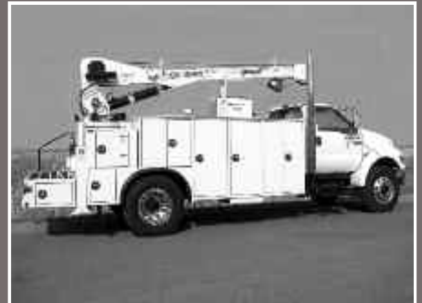
2013 Ford F-750 , 300hp, Feterl body & crane, 40 CFM air compressor, concealed door hinges, LED lights 855-498-0610 J
