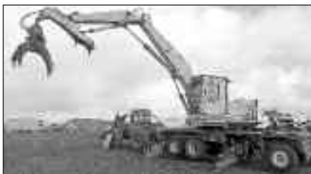
225D Caterpillar Log Loader on 30 ton Pierce SPP carrier, turbo 3208 Cat in upper, 6v92T Detroit w/Allison in carrier, factory mounted Pierce boom & grapple (not adapter), machine is working daily, runs excellent & travels down the road well..... $45,000
