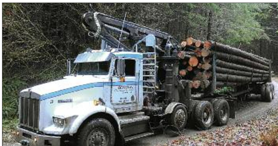
GORDON ENTERPRISES LLC #3, a 1992 Kenworth T-800 with a Cummins N14 mechanical, Eaton 13-spd, Eaton DS402 2-spd rear ends on Hendrickson walking beam, spring suspension. Peerless log gear and Crown 3000 self-loader. Hauling wood from M&M Logging on a thinning job near Randle, Washington.
