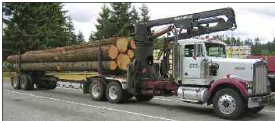
1989 KENWORTH W900 equipped with a 3406B Cat motor, 13-spd transmission, 40,000lb rears and an Olympic 10-ton loader.
