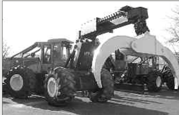
DUAL ARCH TELESCOPIC BOOM SWINGING GRAPPLE mounted on a John Deere 848H skidder seen at the recently completed Intermountain Logging Conference in Spokane Washington.
