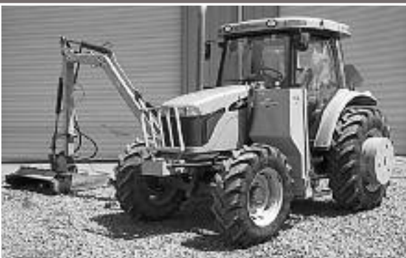
Ex-Government 2009 Challenger MT445B Brush Cutter , A/C & heated cab, 4x4, 105HP, joy stick control Diamond side boom with 4 ft. rotary cutter, 3pt, pto, well maintained $69,500 866-205-7113 R
