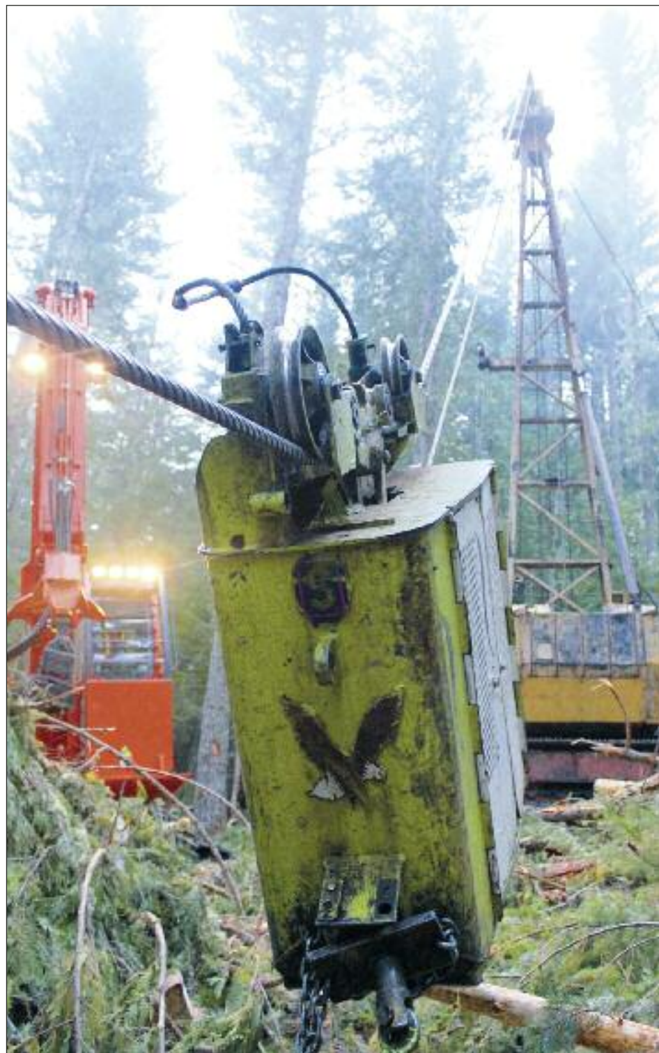
THE EAGLE CARRIAGE of the yarder sits at rest before AnderSons Logging gets started in the morning up near Randle, Wash. at the Gifford Pinchot National Forest.
