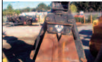
JEWELL MH34B CLAMSHELL BUCKET , 3/4 yard, full rot, 24" wide, Escro teeth, 80mm pins for 200-size..... $10,000
