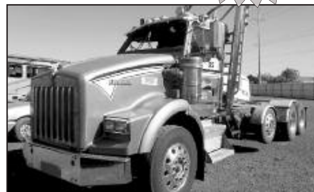
2004 KW T800 Log Chassis, C-15 single turbo Cat, 18 spd./lift axle, Haulmax 46K rears w/locker.GREAT BUILDER/CALL FOR PRICE
