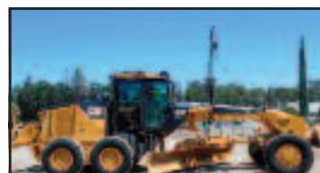
2009 CAT 140M AWD , VHP+, Tier III, 6x6, 14' MB (2' extension available), PB, rear ripper, joy stick controls, beacon, 14:00x24 tires, former county, good condition, 6,300 hours.....$160,000
