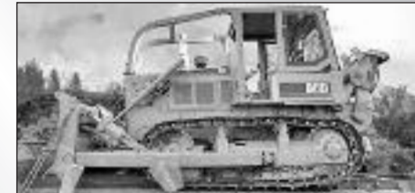
D6D fresh engine with 25 hrs. lights, winch, arch, guarding, $36K
