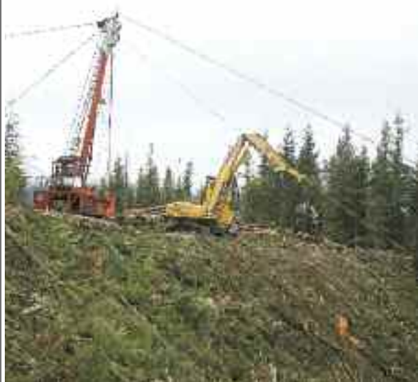
COVER PAGE PICTURE: OUT ON THE JOBSITE, LHH CUTTING AND LOGGING'S 071 Madill Yarder and 200 John Deere With a Wartah Processor get to work.
