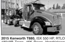
2015 Kenworth T880, ISX 550 HP, RTLO 18918B Trans, 46K Rears, Hendrickson Haulmaxx 46K Suspension, 14.6K front axle, 13.2K Lift Axle, Whit-Log Gear .......
