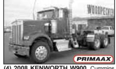
(4) 2008 KENWORTH W900, Cummins 485HP, Jakes, FRO16210C, 13200 Front, HD40k Rears, 3:91 Ratio, Full Lockers, Hendrickson PRIMAAX Susp, 222" WB, All Alum Wheels, Block Heater, Heated Power Mirrors, Full Gauges, 322k—423k Miles \$72,500 ea.
