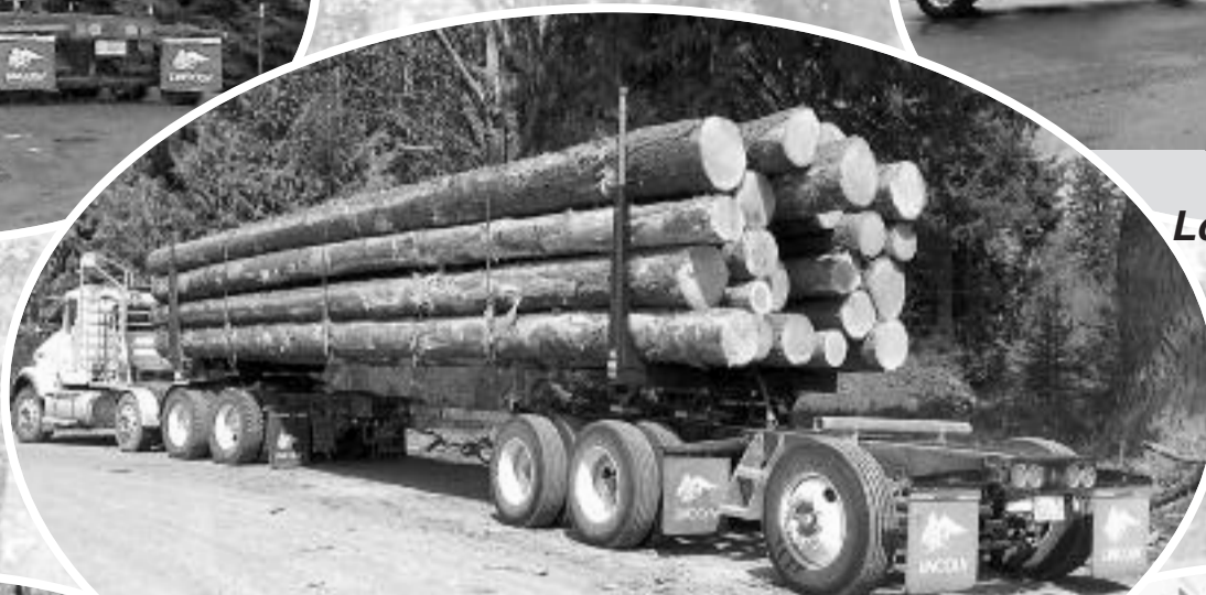
3 Axle Long Log Trailer with Reverse Caster Self Steering 3rd Axle.
