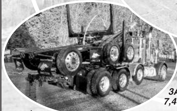
3 Axle Long Log Trailer with Reverse Caster Self Steering 3rd Axle.
