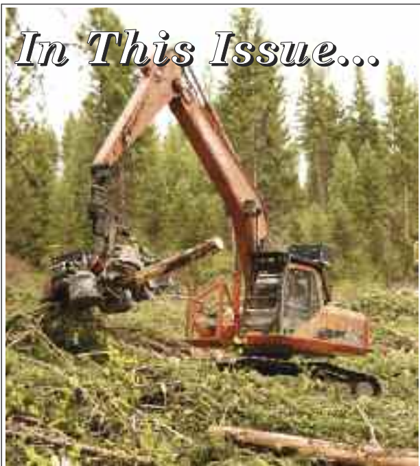
COVER PAGE PICTURE: MATT McMURRAY processing logs with Newton Logging's Doosan 225 with Log Max 7000 dangle head processor, both having 18,000 hours on them. See "It Kinda Got in My Blood" starting on Page 4.
