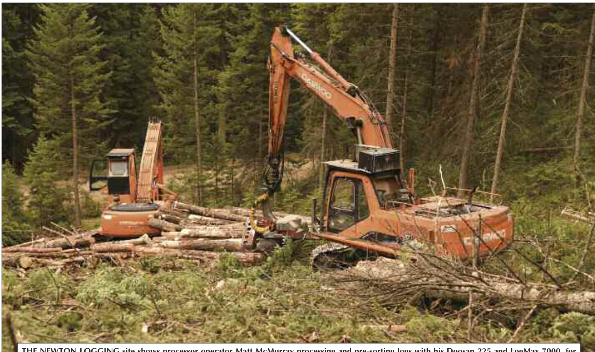
THE NEWTON LOGGING site shows processor operator Matt McMurray processing and pre-sorting logs with his Doosan 225 and LogMax 7000, for Newton Doosan Daewoo 225 shovel with Daewoo boom and grapple with Pierce grapple, operator Todd Boehler. He spent half of his career working on the coast until '99 when he came to Planes, "and I've been logging around here ever since." Boehler just started with Newton, mostly operating loader.
