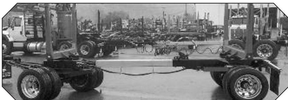
Hubster Trucking , EATONVILLE, WA, Brand New 2015 Whit-Log SPE100 Stick Trailer with Whit-Log Rubber Suspension. Short 8'6" reach to shorten up for loading on back of truck, Lightweight telescopic drawbar, and Much More... Thanks Jim!!
