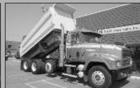
1996 MACK CH613 , E-7 Mack, 427 hp, Jake, 13 speed, 14,600# front, 44,000# rear, tag axle, 16' Sturdyweld Dump Body, plumbed for pup STK. #5113
