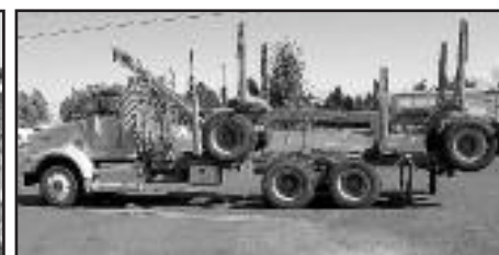
(1) 1992 KW T-800, N-14 Cummins, 15 speed with 2 speed rear ends on pad suspension.
