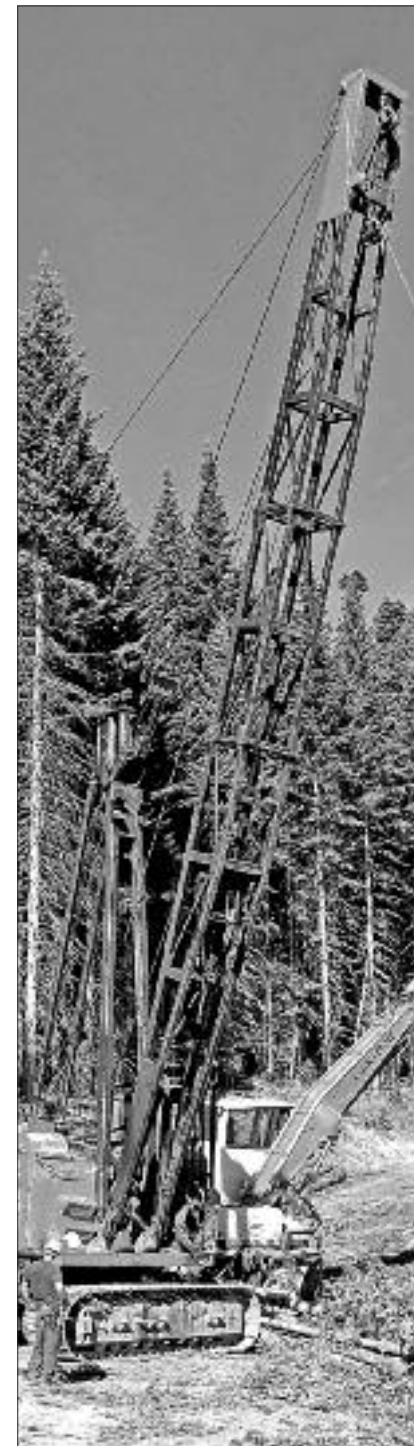
The Link Belt LS 98 with a boom gantry stands tall over the landing for Henderson Logging.
