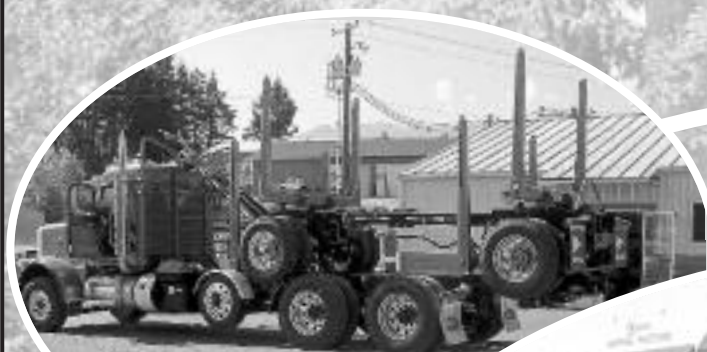
2 Axle Short Log Stick Package with Front Dolly Hop On
