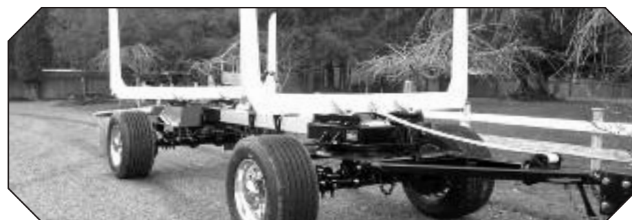
Covey Company, SNOHOMISH, WA, Brand New 2016 Whit-Log SPE100 Lightweight Pup. Custom Turn Table, Front Frame Assy, Drawbar w/ Air Actuated Eye, and Much More... Thanks Todd!!
