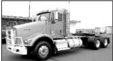
(2) 2011 KENWORTH T800 , Paccar MX 485HP, Jakes, RTLO16913A, 14600 Front, 46k Rears, 3:73 Ratio, Full Lockers, Air Susp, 230" WB, Power Mirrors, Power RH Window, Power Door Locks, AM-FM-CD, 300k & 313k Miles..... $79,500 ea.
