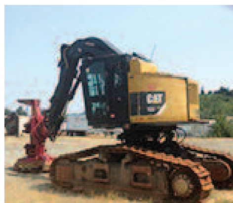
2006 Cat 532 S/N 053200177 Quadco 24" intermittent saw, 360° rotation, 6,000 hrs.
