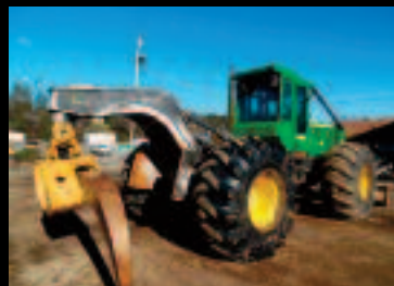
2011 JD 648H, direct drive, single-function boom w/grapple, winch, 2 new/2 very good 30.5 tires, runs & shifts well, 5,590 hours.....$99,500
