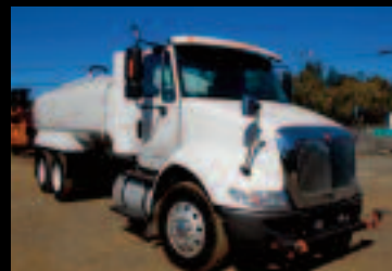
2008 IHC 8600SBA 4,000 GALLON WATER TRUCK, 3 axle, Cummins engine @ 410 hp, 10 speed, air ride, NEW 2015 Randco water system, front, side & rear sprays, hose reel, 8 new drive tires, 489,560 miles.....$57,500
