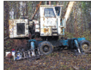
Skagit SJ3R Swing Yarder, 6V53 Detroit Engine, 2 Axle Carrier, 2 Guylines, Radios, 1500' X 3/4".....$65,000
