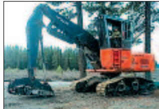
2006 Hitachi 200, 52" Jewell Grapple, 12,200 hrs., New Pump Drive and Rotex, U/C 70%+, New Bottom Rollers, Main Boom and Pins.....$115,000
