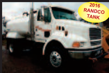
1999 STERLING L8513 2,000 GL WATER TRUCK, 2016 Randco tank, hose reel, hyd fill, CAT eng, manual trans..$32,000
