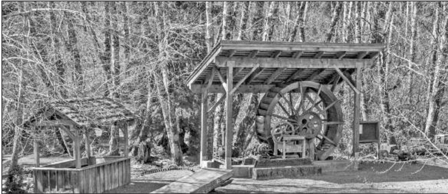
THIS GIGANTIC WATER WHEEL was built by Lee Woodman from his farm on Fishhawk Creek near Jewell, Oregon. It provided electricity for the farm from 1927-37.
