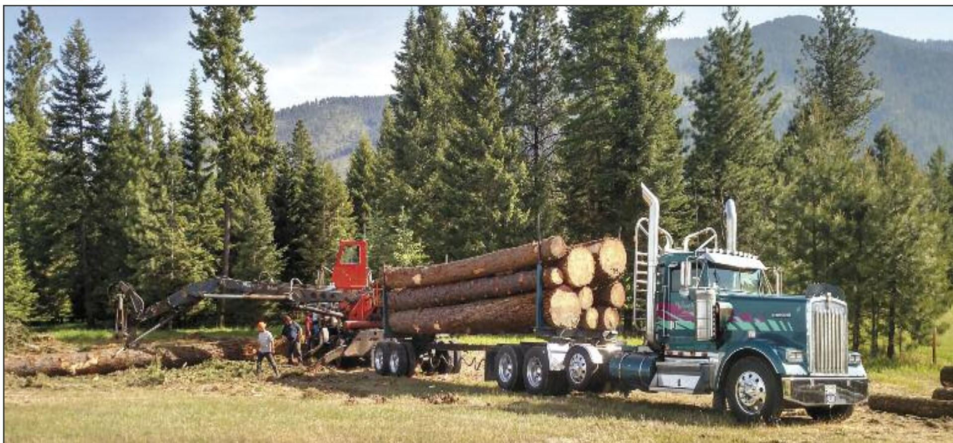
VAUGHT TRUCKING's NO. 9 1999 Kenworth W900L is loaded out on the jobsite. The truck has a Cummins signature series 600-HP motor with an 18-speed transmission and 2001 Alpine gear. (Photo by Kevin Vaught)
