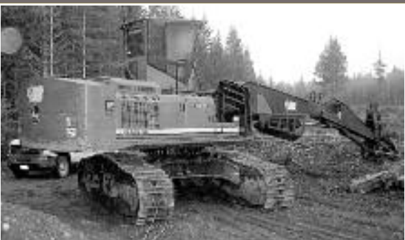
2011 John Deere 3754D Log Shovel , 7,380 Hrs, Great Value, Well Maintained, 43' Log Loader Front, 63" Jewell Grapples, H.D. 450 Size Undercarriage, Side Entry Forestry Certified OSHA, Dual Swing Motors, A/C, Call Tim at (360)532-1485
