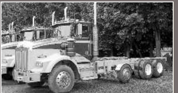
2006 T-800 KW , Cummins ISX (475hp), Jake brake, 18-spd trans.(RTLO18918B), single speed Eaton rear ends (D46-170hp), 4:10 gears w/locker, Hendrickson Haul-max walking beam suspension, 3/8" steel frame, 252" wheelbase, 4-axle truck $55,000 Call Charles Ireland Office: 541-863-5241 - Cell: 541-863-1501 N
