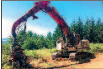
2004 Link-Belt 330 LX Processor with Waratah 624 Super head, 15,085 Hrs., Waratah LogRite Computer, New Rotex Professionally Installed, 60% U/C, Jewel Forestry Cab, Runs Great.....$119,000
