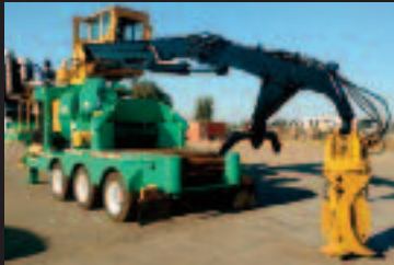
2002 PRECISION HUSKY 66-23, Husky XL-175 loader, CAT 3412, 700/750 hp, Tier I, joy sticks, twin-disc clutch, feed table w/feed chain, cab, 12 new tires, good brakes, fresh oil, new paint, recent injectors, one owner, was working daily, 11,141 hours.....$99,500
