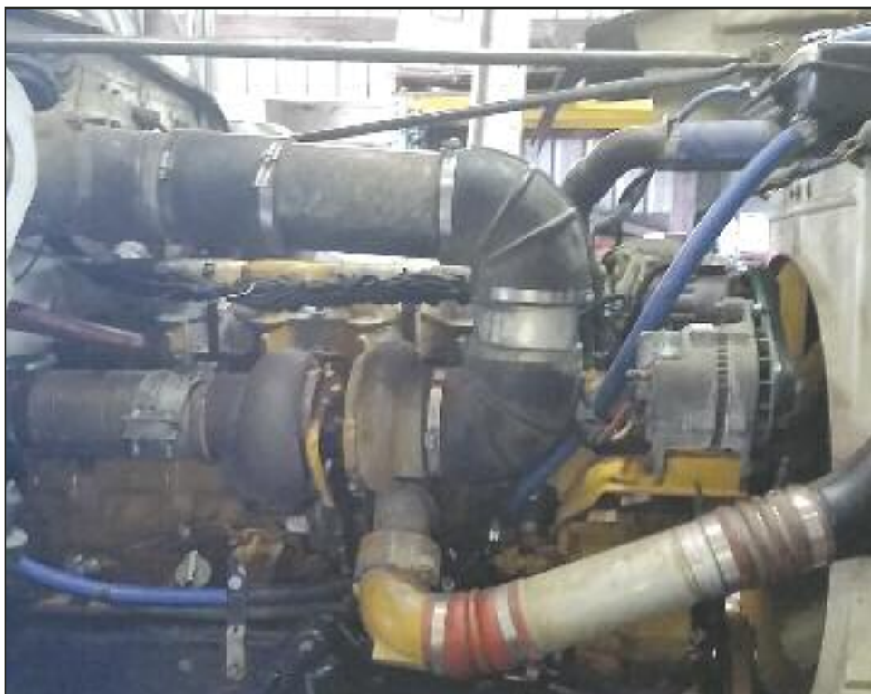
SWITCHING OUT ENGINES In working on his 1979 Kenworth W900A log truck, Todd Stoffel changed the Cummins Big Cam II and put in a 3406E.
