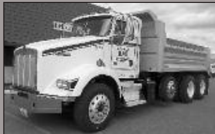
2011 KENWORTH T800 , ISX Cummins, 485 hp, Jake, Fuller 10 speed, 13,200# front, 46,000# rear, air tag, Chalmers susp., full lockers, 16' dump body STK. #5229
