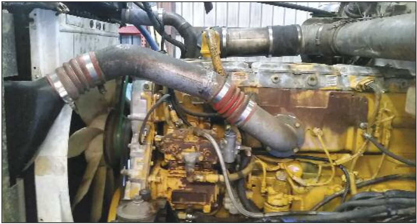
SWITCHING OUT ENGINES In working on his 1979 Kenworth W900A log truck, Todd Stoffel changed the Cummins Big Cam II and put in a 3406E.
