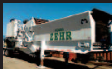
2005 ZEHR HG4000 GRINDER, early Diamond Z, 2009 CAT C27, Tier II, 1,050 hp, remote, stacking conveyor, 8 NEW tires, good brakes, twin-disc clutch, hamermill approx. 62" x 17", approx. 85,000 lbs. w/o tractor.....$129,500
