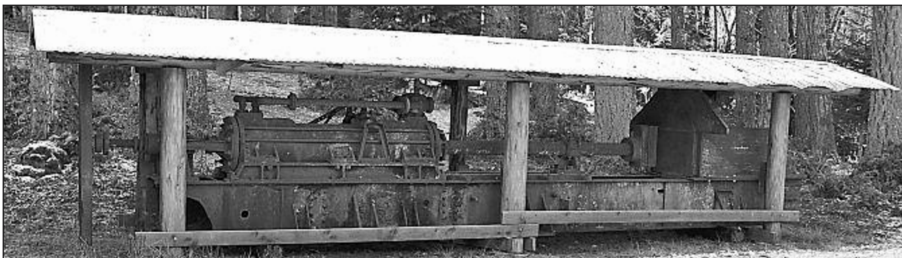
Another large, interesting piece in Fred's collection is this steam-powered wood splitter from the old St. Helens Pulp and Paper plant. This mammoth machine was built by Portland Ironworks.
