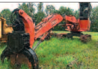
1999 Madill 3800B LOG LOADER, 8200 hrs, Rebuilt 8.3Cummins, Good U/C, 63"Jewel Grapple, FRESH hydraulic pumps, Automatic greaser & Fire Suppression.....$165,000
