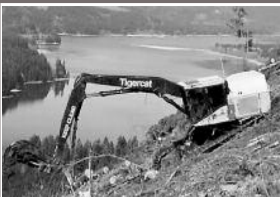
Tiger Cat 855c with Waratah FL85 series 2 felling head, grouser ext. and tow point. Call 253-405-3586 for more information and pricing. A
