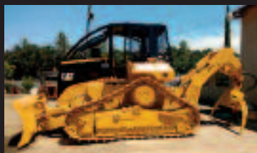
1997 CAT 527 24,069 Hours, fixed-boom-grapple, No winch, Prolenc snubber, recent engine work, new CAT rails, pads and idlers, 7-roller track frame, good condition for hours .....$132,500
